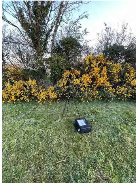
Figure 5: Attended noise monitor setup.
